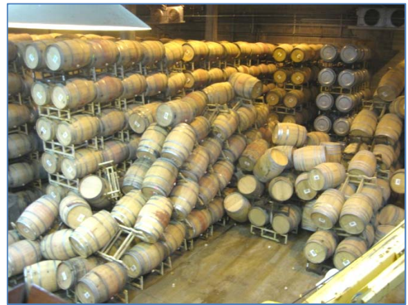
Wine barrel collapse at a Napa winery.
